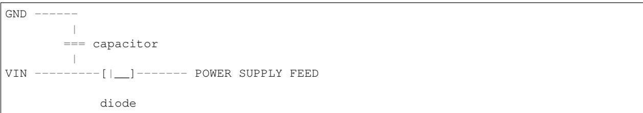
The above solution can reduce but not eliminate transient voltage spikes. A more decisive way to deal with transient voltage is to use diodes in opposition. This technique reduces the short duration electrical spikes can occur because of power shortages, power transitions in other large equipment on the same power line or lightning strikes.
